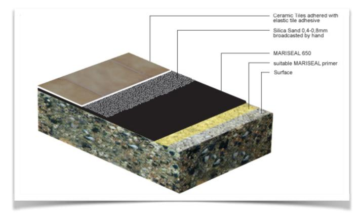
Immediately before the application of any component of the system, the substrate shall be dry, with any remaining dust or loose particles removed using clean, dry, oil-free compressed air, industrial vacuum, cloth-wipe or a combination.
